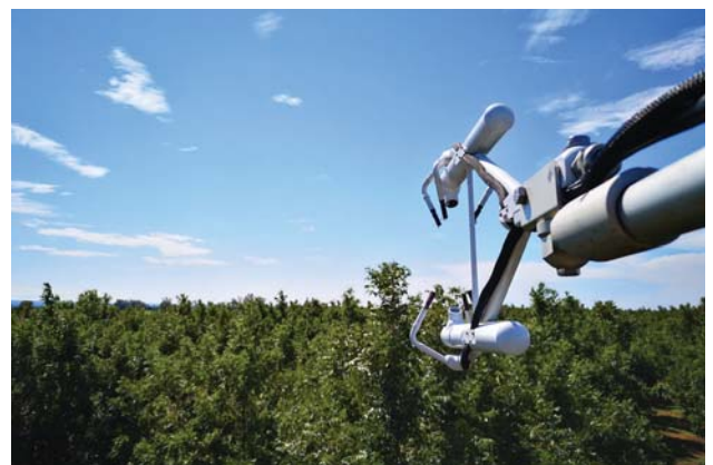
The infrared gas analyser and 3D sonic anemometer which forms part of an eddy covariance system. These instruments aid in the determination of water vapour and CO 2 fluxes, which when combined with other measurements can be used to estimate evapotranspiration.
