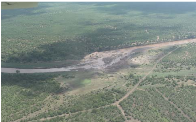
The Kanniedood Dam before, during and after demolition in 2018/19. The dam was removed completely after the wall was breached by flood in 2013, causing the river to open a new channel bypassing the dam wall on the southern bank of the Shingwedzi River.
