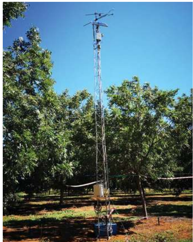
The eddy covariance tower in the 15-year-old mixed cultivar pecan orchard outside of Jan Kempdorp, which determines total water use or evapotranspiration of the orchard.
