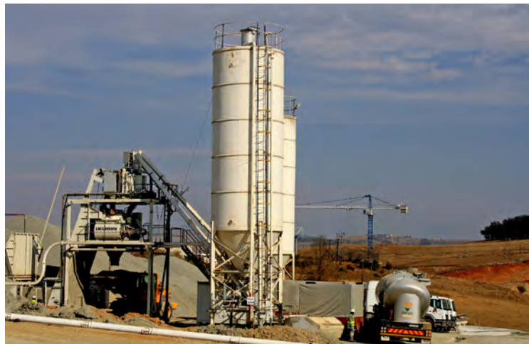
Top left: The Spring Grove batch plant. Around eight days' worth of material is stored on site.
