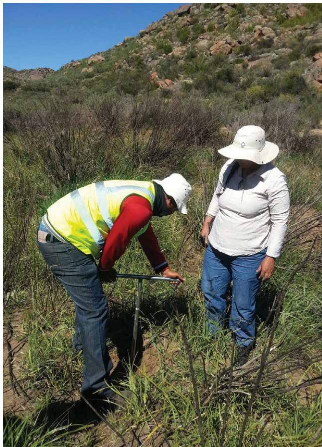
A dipwell is installed, by first drilling a hole with an auger and sinking a dipwell into it for long-term monitoring of the water table.
