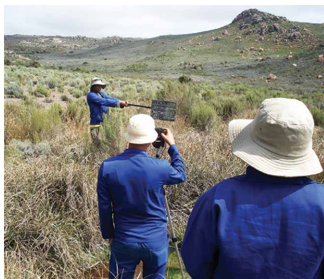
Fixed point photography: Photos are taken in four wind directions, from the same point. Information on the specific point is indicated with the small, black board.
