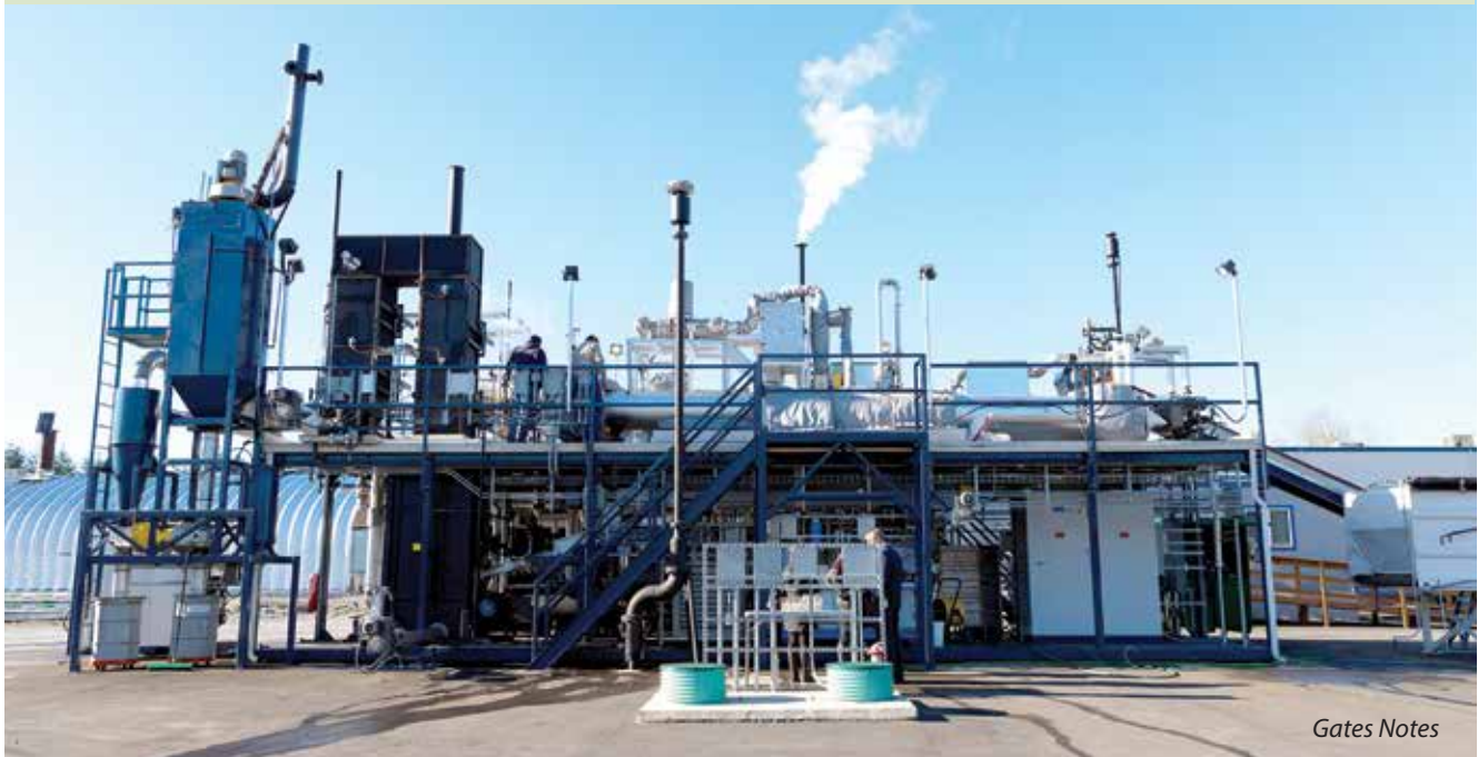
The Omni Processor is being piloted in Senegal, where it will convert solid waste from pit latrines into drinking water.
